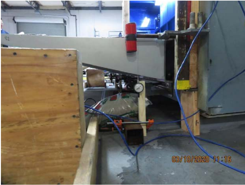
7700 Series Sunshade Prior to load testing
