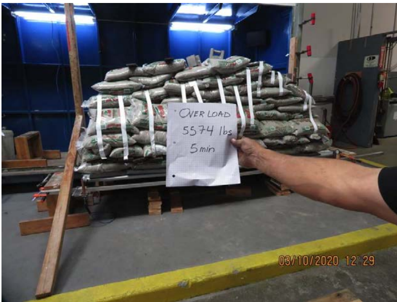
7700 Series Sunshade Shows the Overload testing
