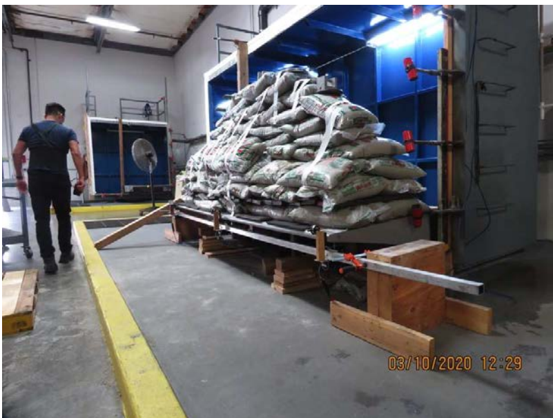
7700 Series Sunshade Shows the Overload testing
